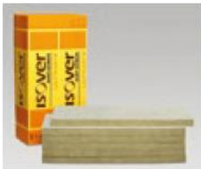
U Protect Slab 4.0 V1 Slab: 1200 x 600 mm Facing: glass tissue
